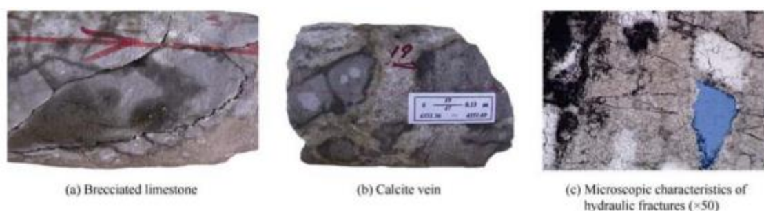
Figure 21 - The features of hydraulic fractures caused by overpressure in the Carboniferous reservoirs of the Kenkiyak pre-salt formation.
